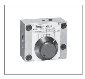
This valve controls flow by changing the cross-sectional area through which fluid flows. Since it incorporates a pressure compensation mechanism, the flow is kept constant even if the pressure varies at the IN and/or OUT port.
