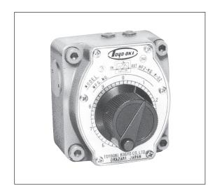
This valve controls flow by changing the cross-sectional area through which fluid flows. Since it incorporates pressure compensation mechanism and temperature compensation mechanism, the flow is kept constant regardless of the pressure variation at the IN and/or OUT port and the viscosity variation due to temperature change.
